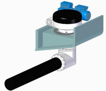
(Showing Standard Steel Bushing – Diameter 217MM)
